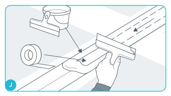
Fill all joints with an appropriate filler along with a paper strip. When the filler is dry, use sandpaper and make a smooth surface between the boards. Do not overlap the paper strips.
