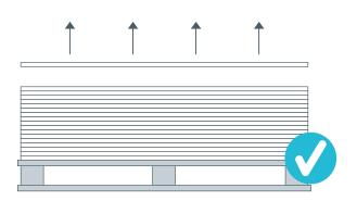
If the board is pulled off the stack, the acoustic tissue on the backside might get rolled of the board. This might give some issues with the level between boards during the installation.
