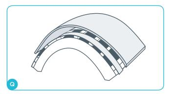
Carefully lift up the plasterboard when it is 100 % dry. The curved plasterboard must be installed maximum 2 hour after it is removed from the form. If not – it will assume its original shape.
