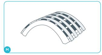
Build a template so it will be possible to curve the wet plasterboard around the template, in the specific curved radius. Radius from 2.2 meters to 1.2 meters use wet bending.
