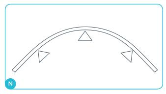
Use clean water – if possible (use also a little part of rinse aid (surfaceactive agent for a dishwasher)) – this will help the water to go into the gypsum core more quickly. Water must be applied on the side of the plasterboard closed to the centre of the radius.
