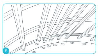
Where there is a connection between the short edges of the BIG Curve, it is important to place the cross channels with a centerdistance of 150 mm. To secure a smooth curved transition between the BIG Curve boards. See also illustration I.
