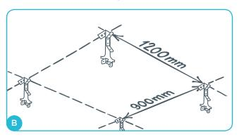
Plan out where to place the adjustable hangers GK 26-01/GK 27. Fix the adjustable hangers using apppriate fasteners. Hanger center distance = 900 mm. Main channel center distance = 1200 mm.
