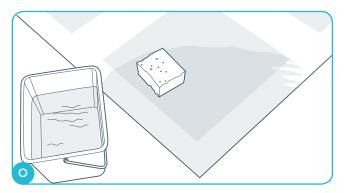
Place the plasterboard on an even floor or a table. Applied water with a sponge on the plasterboard. Only a small amount of water the first time. Apply more water after 2-5 minutes (continue to apply water for 15-20 minutes in total). Avoided water inside of the perforation.
