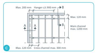
The first hanger should be place with a maximum distance of no more than 200 mm from the wall. The center distance for the main channels (GK1) is 1200 mm. The first main channel (GK1) should be placed no more that 120 mm from the wall. See detail drawing on page 4, for description of section A-A and B-B.
