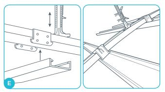
Place the jointing plate GK 22 on top of the main channels. Then push the cross channels (GK 1) up into the jointing plate. Cross channels are installed with a centerdistance of 300 mm.
