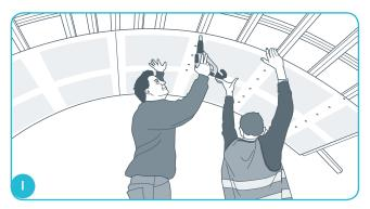
Installation of the boards on the grid system, must be done with an even amount of pressure applied to the boards (push very slowly). Place the screws according to the fixing template on page 5. The board must be curved along its length.
