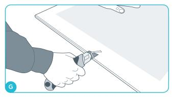
BIG Curve has only taped edges on the long sides. On the short sides, it is important to make a bevelled edge with a knife so more filler can be applied in the connections between the boards.
