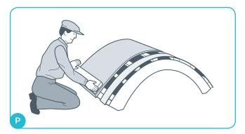
Carefully lift the wet plasterboard and place it on top of the template. Apply pressure on the edges with a flat, wooden plank or steel stud and fix the stud with a clamp until the gypsum board is 100 % dry.
