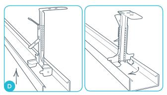
Lift the main channels (GK1) up and attach the GK26-01 hanger to it, by twisting the hanger into the main channel.
