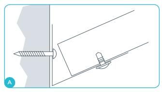
Fix twisted steel sheet VPB 50/50 to a wall. Use screws with a pan head and fix them to the wall with a center distance of 400 mm. See detail drawing on page 4, section A-A and B-B.
