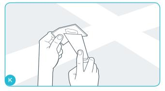
Filling the screws, use appropriate filler. Keep using filler and sandpaper until surface of the board is smooth.
