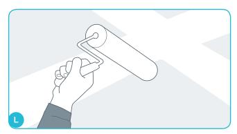
Painting the BIG Curve is done with a shorthair mohairroller. Avoid paint in the perforation. It is not allowed to spray paint BIG Curve, because of the risk of getting paint on the acoustic tissue. If paint is applied to the acoustic tissue, this will strongly reduce the BIG Curves acoustic performance. The BIG Curve is primed and then painted twice.
