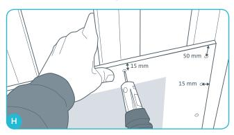
The board must be fixed to the steel system with special Gyptone QSC25. All short edges must be supported by the steel system.
